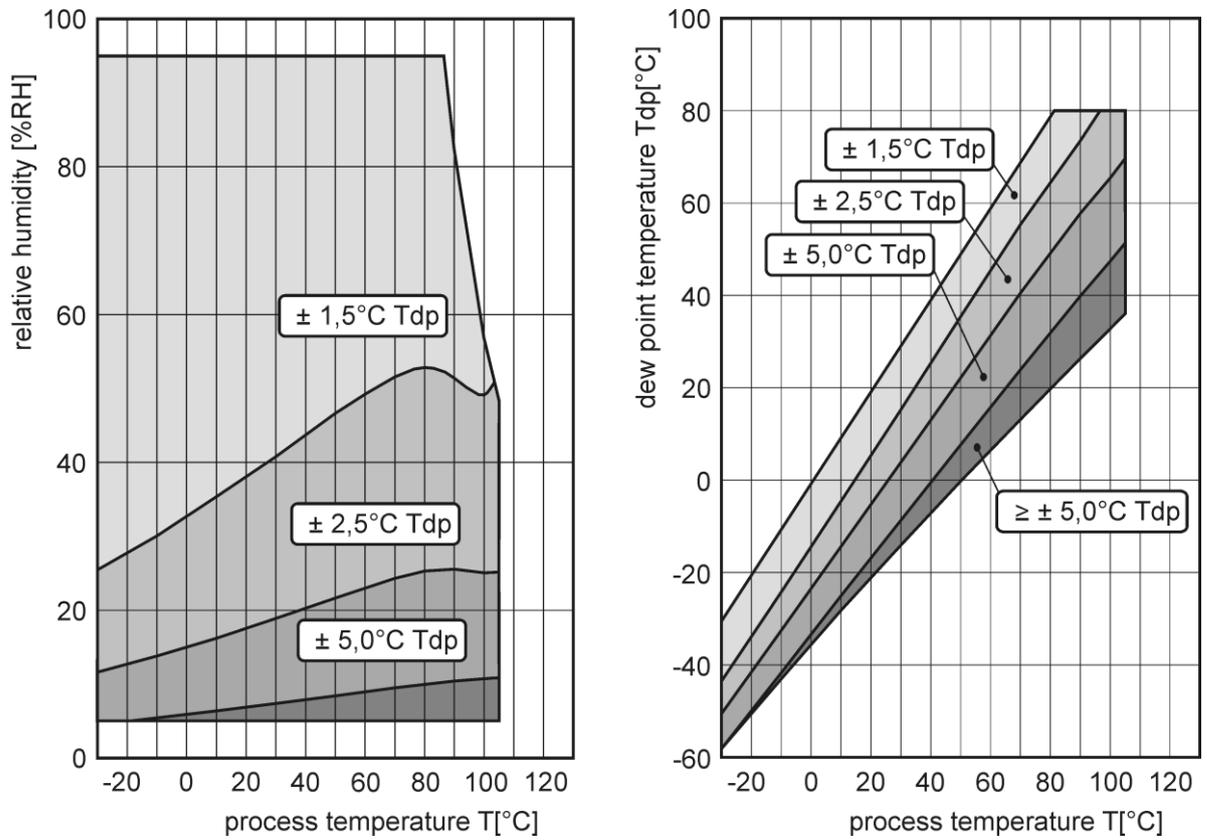
Accuracy of computed absolute humidity for compressed air measurement up to 25 bars.
